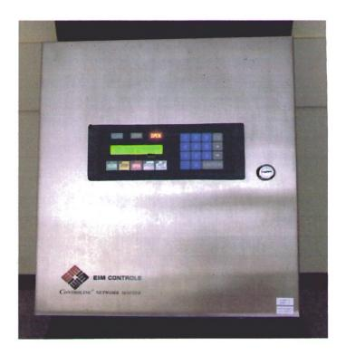
Enclosure is NEMA/EEMAC Type 4X IEC IP66 wall mount with sealed rear mounting holes or mounting brackets. Includes (5) five NEMA 4X liquid tight strain relief compression type cable entries or will accept ½ inch conduit. Separate entries are provided for power (1), actuator networks (2) and host links (2).
