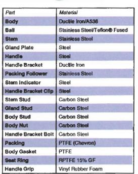
This patented Ductile Iron Ball Valve has been engineered to replace any plug valve, carbon steel ball valve, or gate valve.
