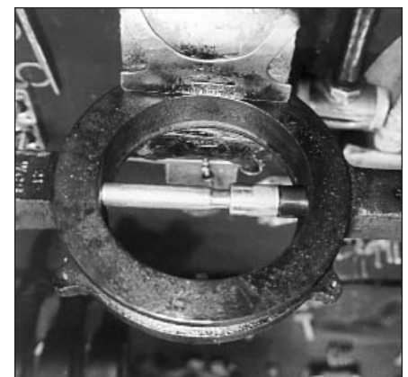
Figure 6 – Shows partial insertion of the stem bearing.
