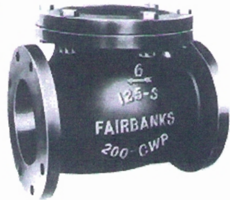
Fig. 0702/0702AI Swing Check Valve 2"-24" Flanged 125 PSI SWP 200 PSI CWP Available in All Iron sizes 2"-12" Conforms to MSS SP-71 Type I
